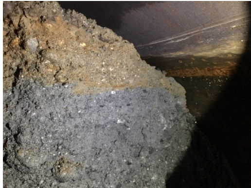
Figure 10 Soil inside leading pipe segment showing alluvium/recessional soils (brown) underlain by dense glacially overridden soils (gray).
