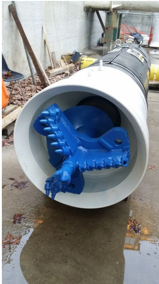
Fig. 13 – cutting disc with auger soil removal
