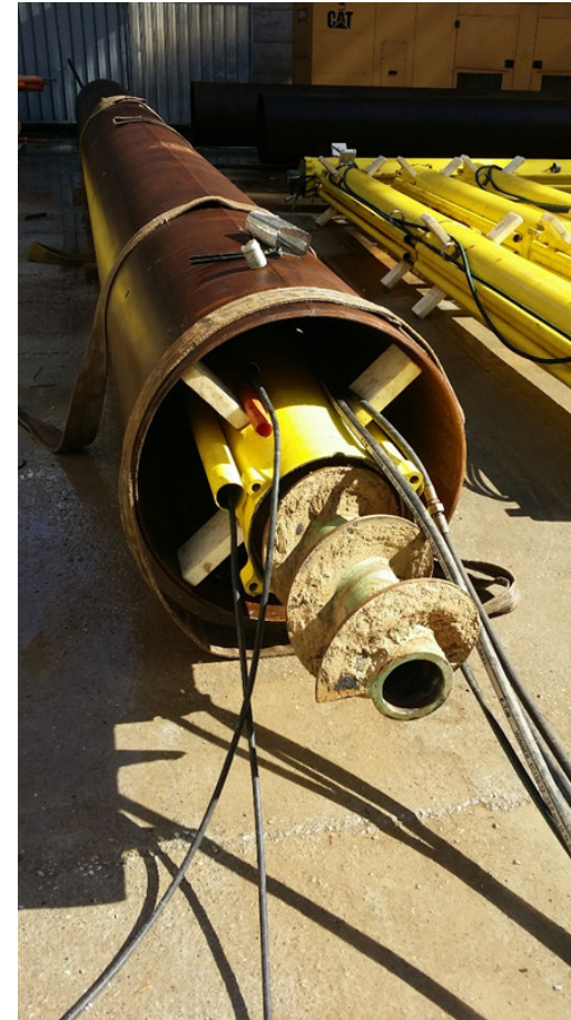
Fig. 13 – cutting disc with auger soil removal
