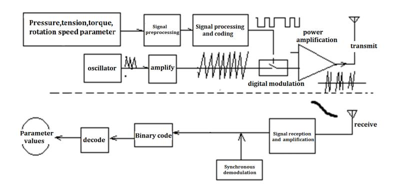
According to the method of parameter detection, the modulated transmission method is used. After receiving the signal, the receiver will amplify, filter and shape the signal to obtain the preprocessing signal. Part of the circuits demodulate the signal and restore the modulated signal to obtain the parameters in the hole.
