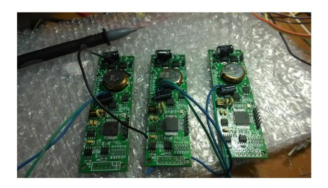
In order to meet the installation requirements, the size of the circuit board was controlled at 100mm\*30mm (3.937inch\*1.181inch).
