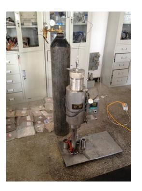
Special pressure sensors were put into the autoclave for pressure test, and the pressure was stabilized for 30min after the pressure was added to 6Mpa (870psi).
