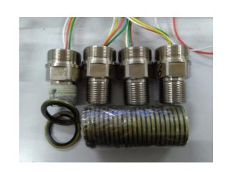
Considering the limited space for installation, a customized pressure sensor is adopted to further compress the circuit board space, remove the outer cylinder, and protect the circuit board with high-strength sealing glue.
