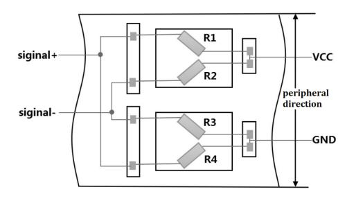
When measuring torque, the strain gauge should be paste along the axis of the measurement part at a 45° angle and connected to the full-bridge circuit for measurement.
