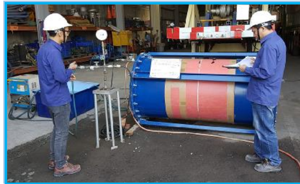
inner Pressure test ( \leq ID 4% under 0.3 Mpa)
