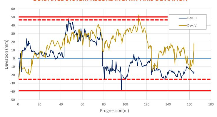
Deviations recorded by the TBM are within the limits provided by ATVA 125 for drains and sewers (gravity flow)
