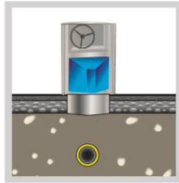
Creating the core bore with core drill unit by TRACTO-TECHNIK
