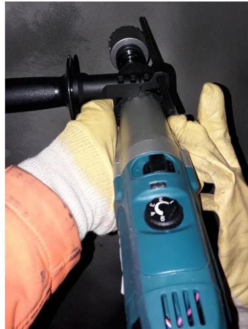
Tear test on grout for wells recovery
