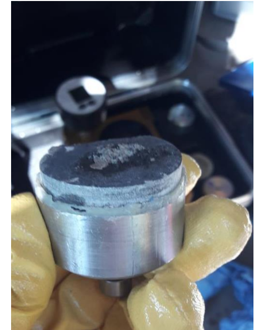
Tear test on grout for wells recovery
