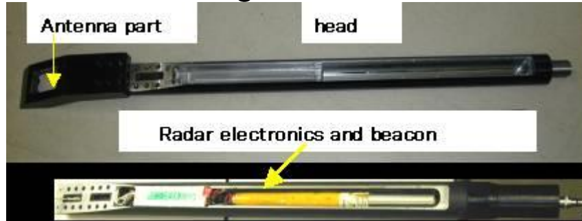
(a) GPR set on head of horizontal boring machine
