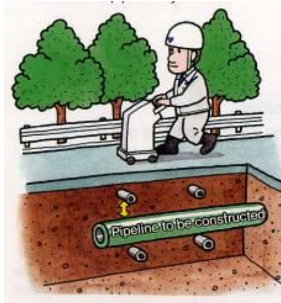
(b). Survey before horizontal drilling
