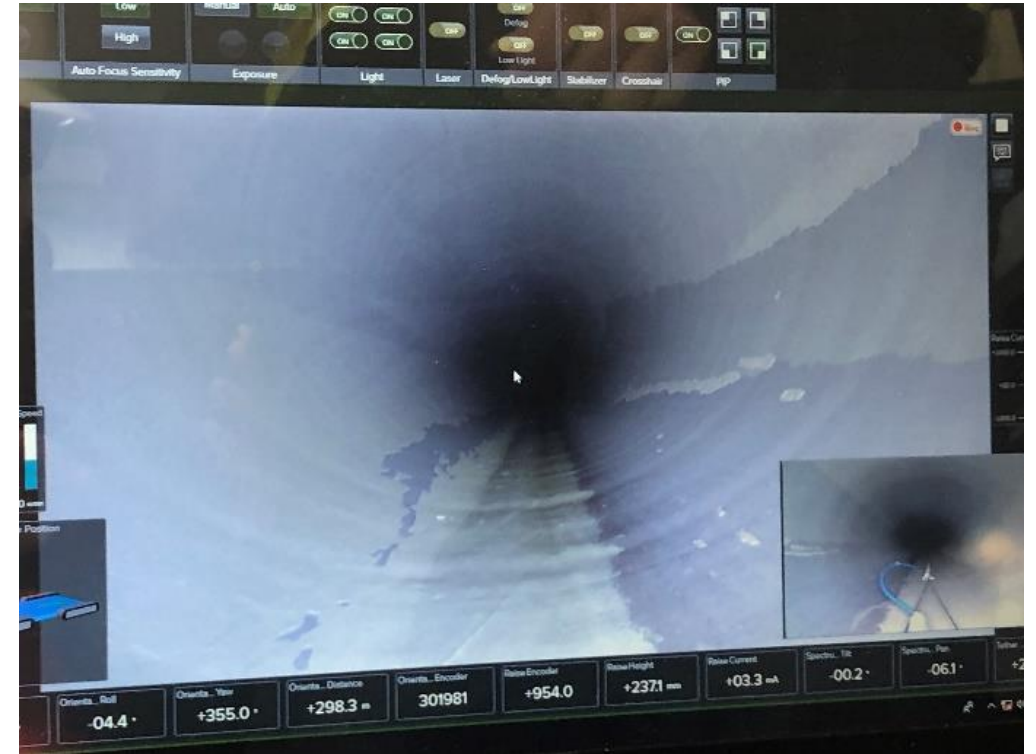
CCTV inspection in a 2100mm Steel Pipe with no water
