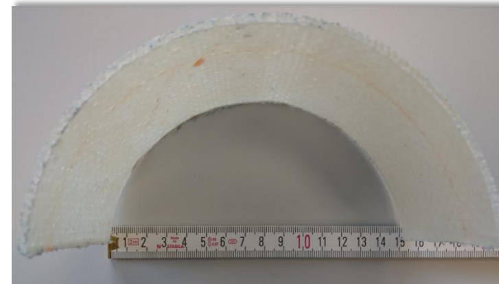
Seamless invertable GRP Liner DN150, e_c \approx 2,4\text{mm}
