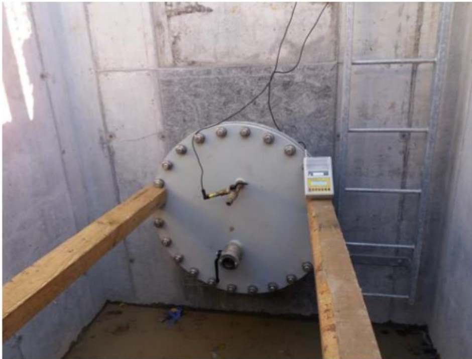
The set up for the hydraulic pressure test
