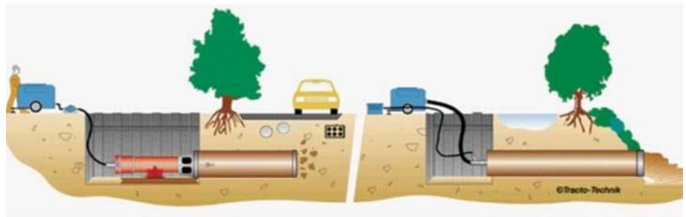
Typical Pipe Ramming Uses Diagrams by courtesy of TTUK Ltd.
