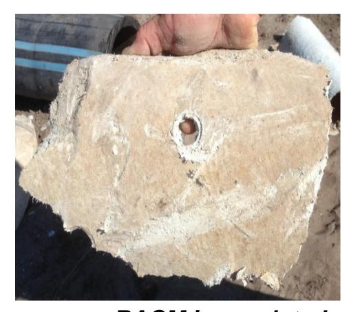
RACM is regulated AC pipe that can be further reduced to powder by hand
